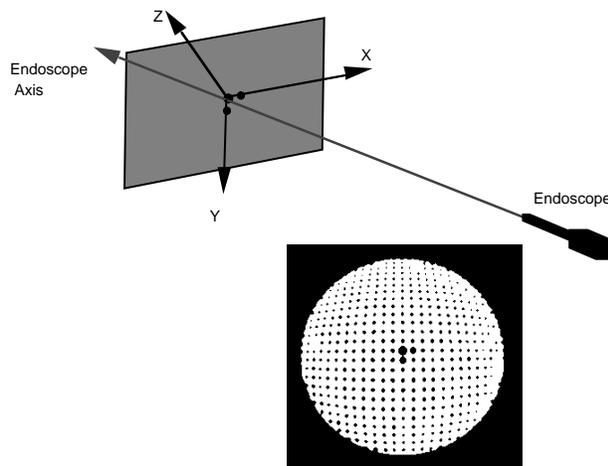
The detected image plane represents the observed image plane actually visible through lenses with radial distortion. This detected plane is identified by computer vision algorithms (first the center dot and the directions of the X-Y axes are determined, then by a sorting algorithm each calibration dot is addressed by an index). The grid plane is defined by the original flat reference grid by setting up the right orientation with a (linear
