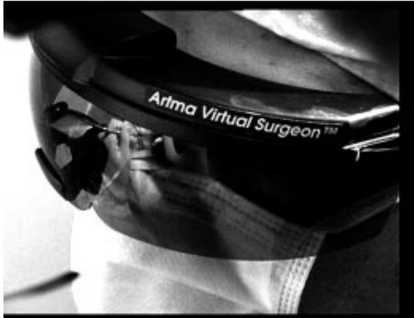
**The live video image fusion concept eliminates the need for additional computer monitors for stereotactic navigation information.** The integration of the Head-Up display was demonstrated as work in progress.
